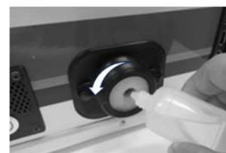
Inject the lubricant while rotating the part
