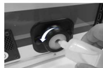
Inject the lubricant while rotating the part
