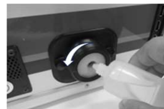
Inject the lubricant while rotating the part
