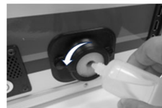
Inject the lubricant while rotating the part
